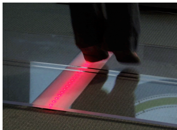
figure 6. jump sensing board with pressure sensor and led light strip
